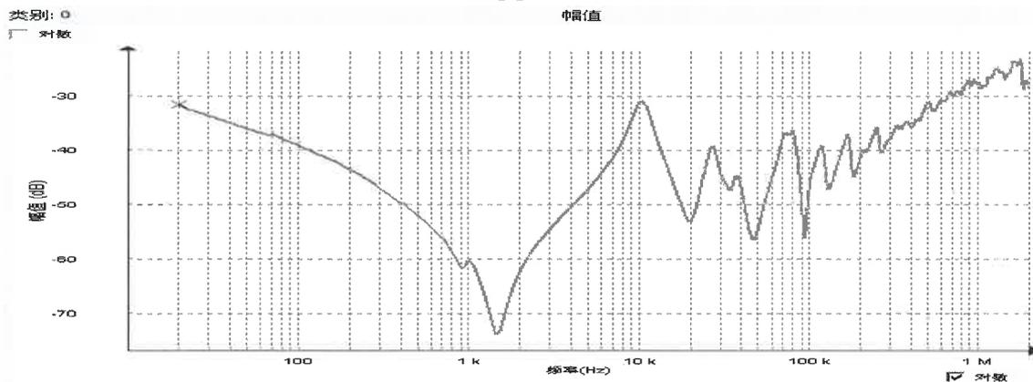
LV windings frequency response curve after short circuit test
