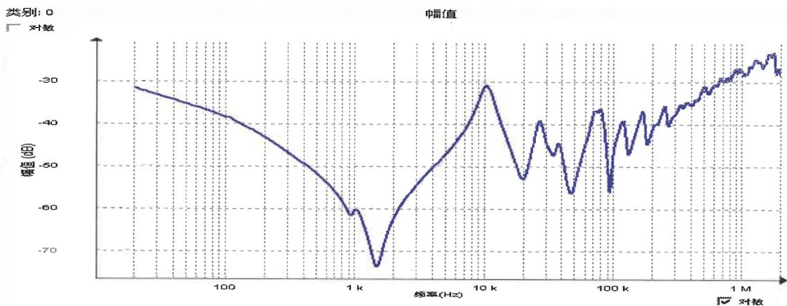
LV windings frequency response curve before short circuit test
